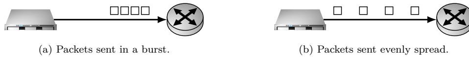
FIGURE 2.4: Qualitative comparison between a traffic burst and evenly spread packets. Adapted from [20].
