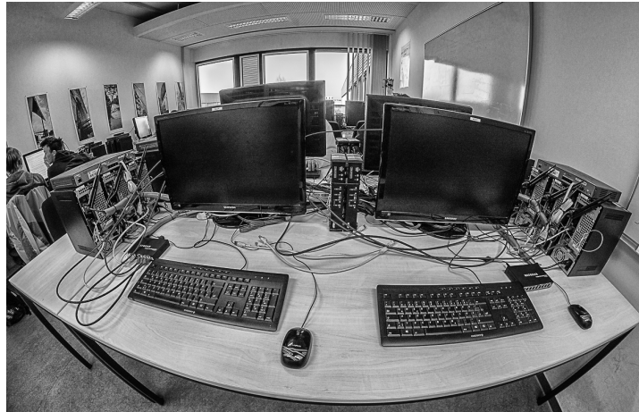
Figure 2.1: Workspace for students of the iLab course called “iLab Isle”: Students typically work in groups of two, so each each isle offers two full workspaces side by side. To be able to simulate complex network setups each isle also has six special iLab PCs with five ethernet ports each and two Cisco routers.
